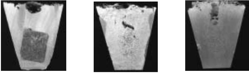
Figure 2: Some scanned images of the cast samples for 85% Mn-containing 200 gram mini-tablets. The tablets were extracted after 60 seconds, 120 seconds and 240 seconds after addition.
