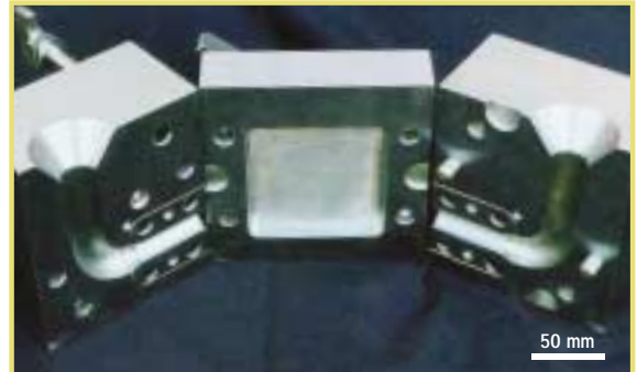
Figure 1 – Photograph showing the three-part steel permanent mould used in the experimental work.
